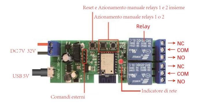
**RELAY –**Relay for 10A AC/DC NO/NC
