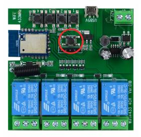
In the center of the board is the reset button. If you hold down the reset button for 5 seconds restore factory settings and the device goes into standby mode
