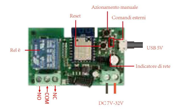
RELAY –Relay for 10A AC/DC NO/NC NETWORK INDICATOR –2.4GHz WiFi status blue LED. Flashes quickly when the device and waiting for app setup. MANUAL OPERATION –Buttons for direct control of relays RESET–Press 5 seconds to reset USB 5V –MicroUSB 5VDC power input
